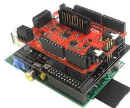
FIGURE 3.4: eHealth shield on Raspberry Pi
