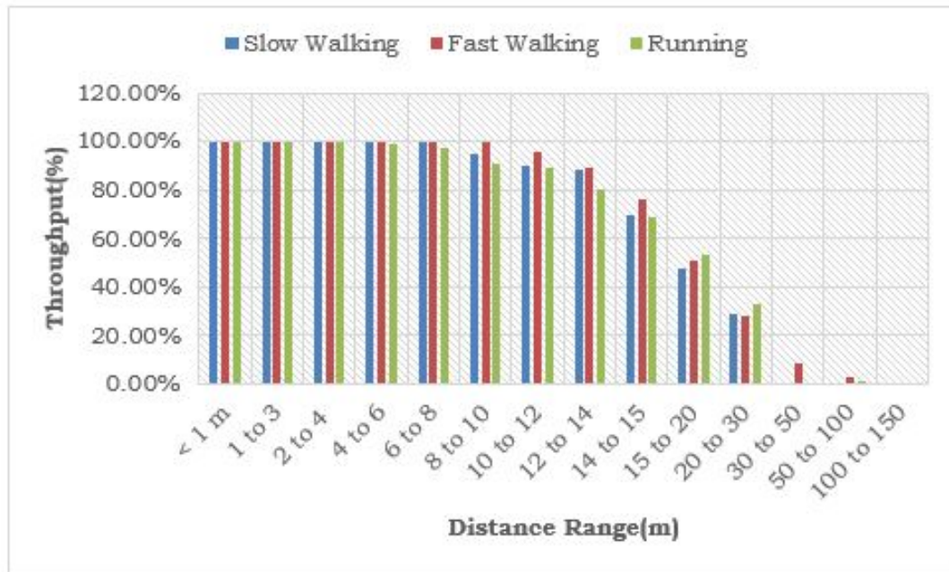
FIGURE 4.17: IEEE802.11 Throughput experiment one
