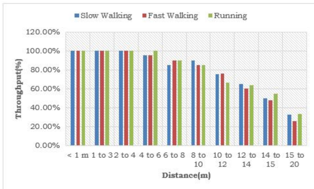
FIGURE 4.15: IEEE802.15.4 Throughput experiment one
