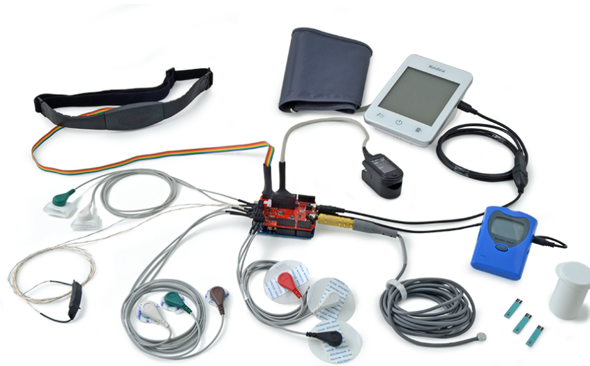
FIGURE 3.1: The e-Health sensor kit with sensors attached.
