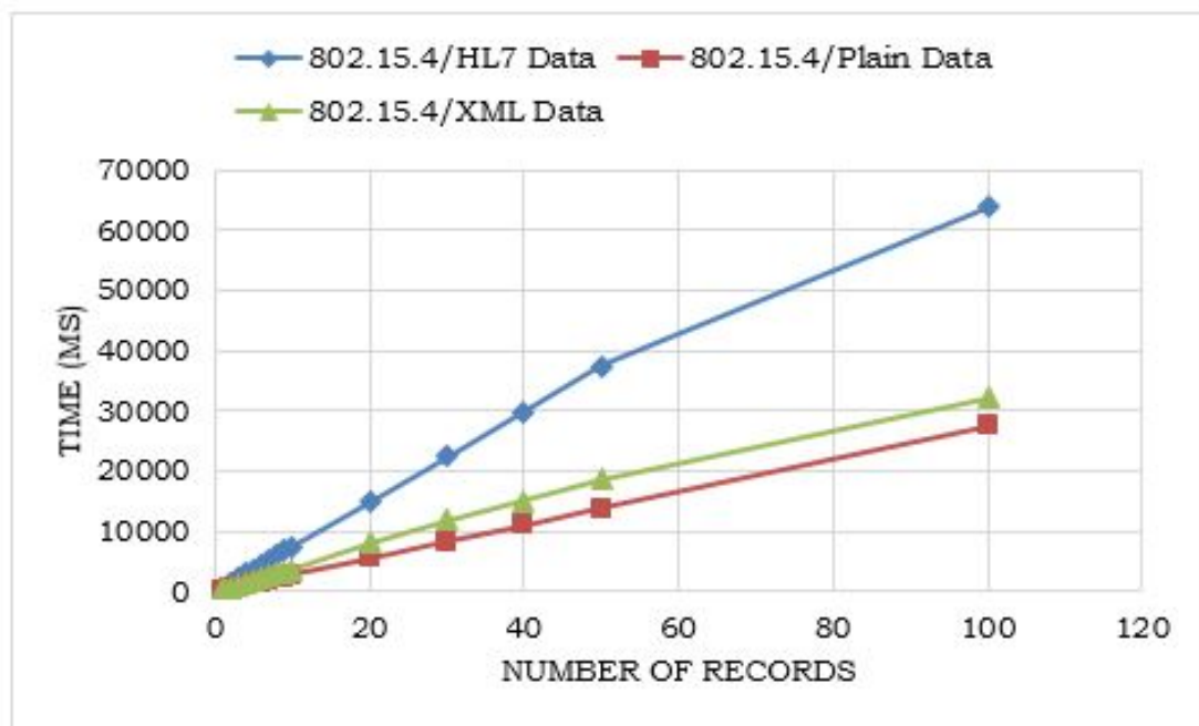
FIGURE 6.5: 802.15.4/ZigBee Single hop Data delay Overhead
