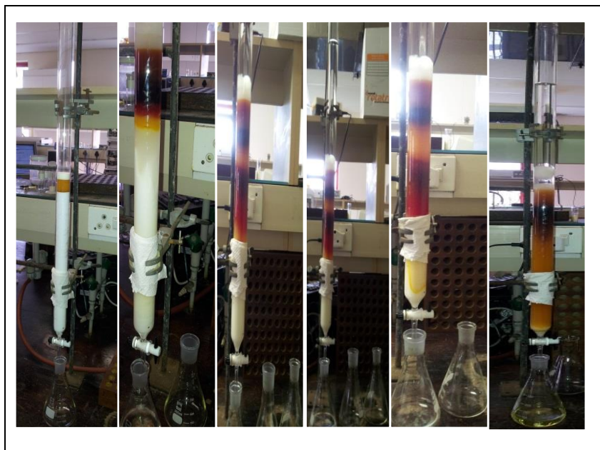
Figure 4.2: Column chromatography setup (7 X 30 cm, 500g silica gel) for collecting fractions which were screened using HPLC. Each colour in the column represented different fraction.
