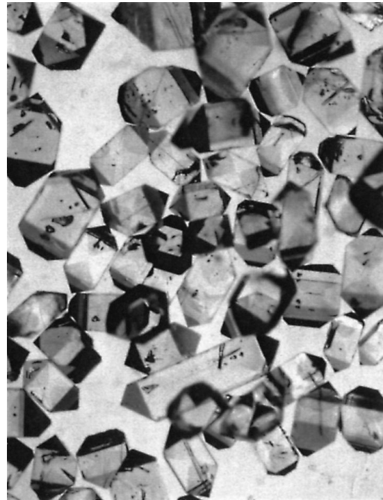
Figure 3. Photomicrograph of separated zircon crystals. Most crystals contain solid and fluid inclusions. Those selected for analysis were free of inclusions. Field of view, 3 mm.
