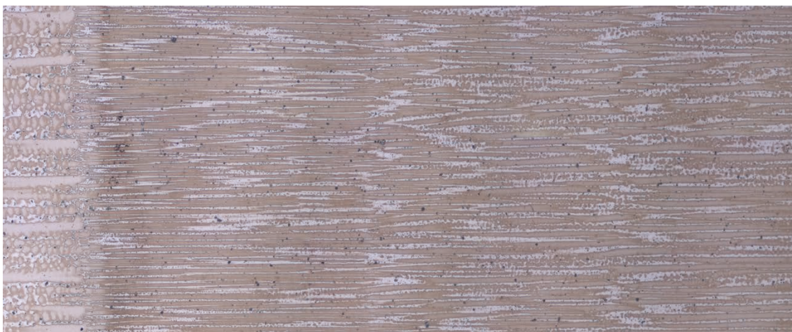
Fig 3- 91: Dendrite width evolution from Fusion line, sample G91
