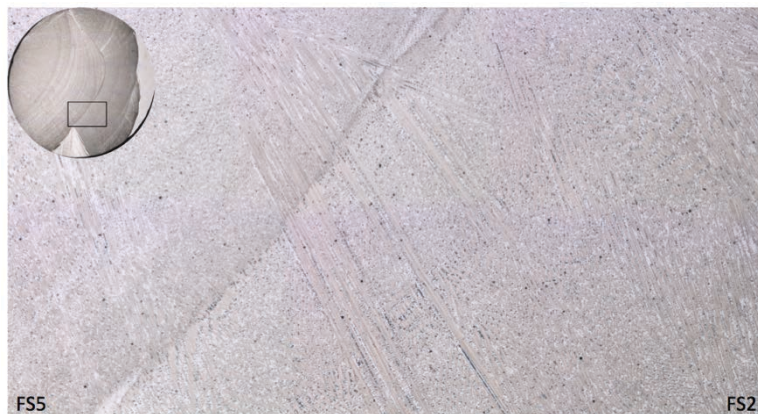
Fig 3- 100: Large grains crossing FL between weld bead FS2 and FS5, sample G156
