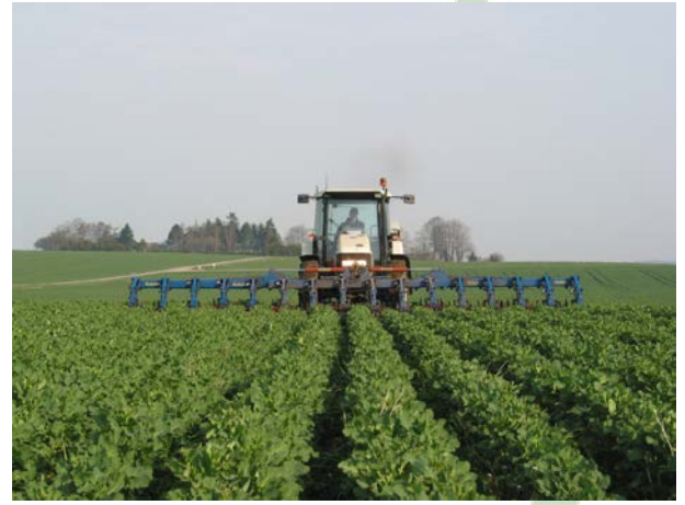
Inter-row hoeing in late April using a front-mounted hoe for manual steering
