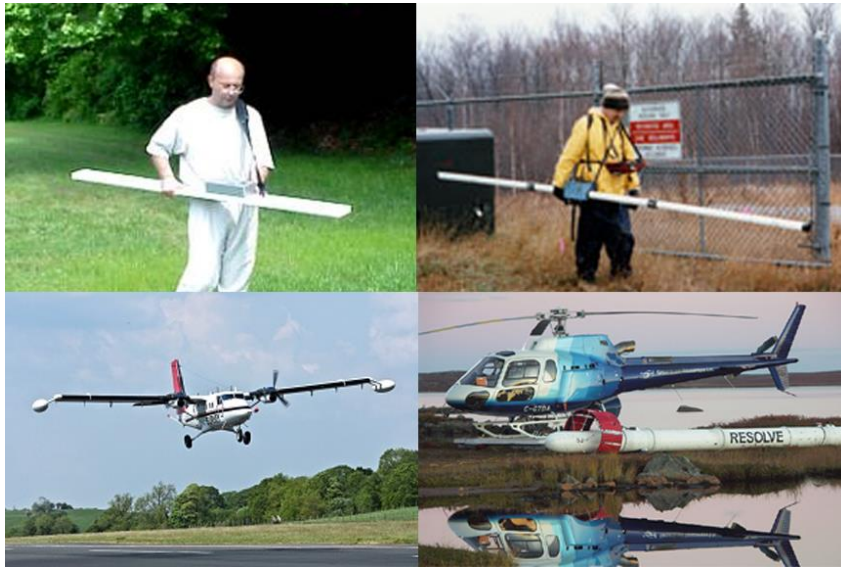
Figure 2.10: Examples of ground and airborne FDEM systems. At top left is the GEM-2 from Geophex Ltd., top right is the EM-31 from Geonics Ltd., bottom left is the SGFEM fixed-wing system from Sander Geophysics, and at the bottom right is the RESOLVE heliborne system from CGG.
