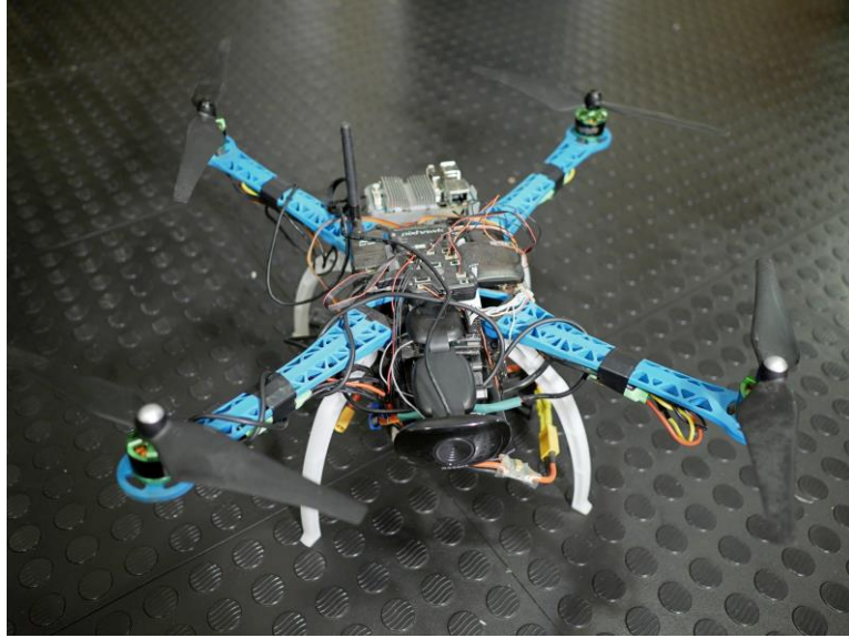
Figure 5.14 – S500 Hobbyking UAV with a developed auto-landing system
