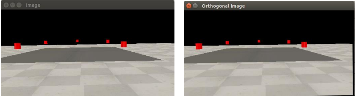
Figure 2.8 – Camera image and virtual orthogonal image for \alpha = \alpha_{ship} - \alpha_{UAV} \approx -0.01rad, \beta = \beta_{ship} - \beta_{UAV} \approx -0.02rad
