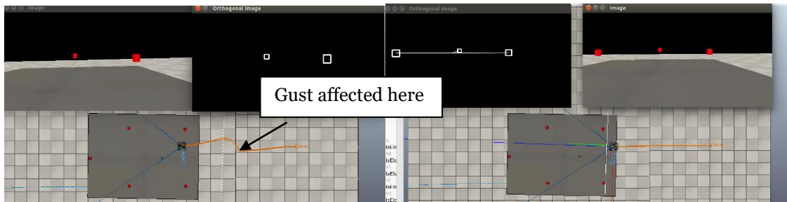
Figure 5.9 – Perturbations during landing mission: a) gust affecting the UAV trajectory; b) wind affecting the UAV trajectory
