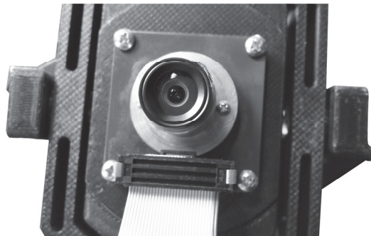
(b) 2DOF POM mobile platform with image sensing PCB attached.
