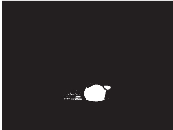
Figure 6.3: Thresholded image at optimal value obtained via manual thresholding.
