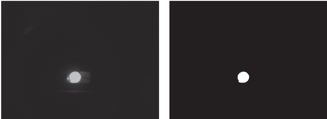
(a) Improperly diffused IR LED with filter in front of the image sensor. (b) Filtered IR light upon receiving thresholding of the image sensor.
