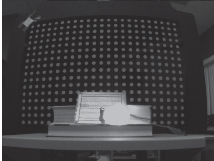
Figure 6.1: IR LED experiencing poor diffusion.
