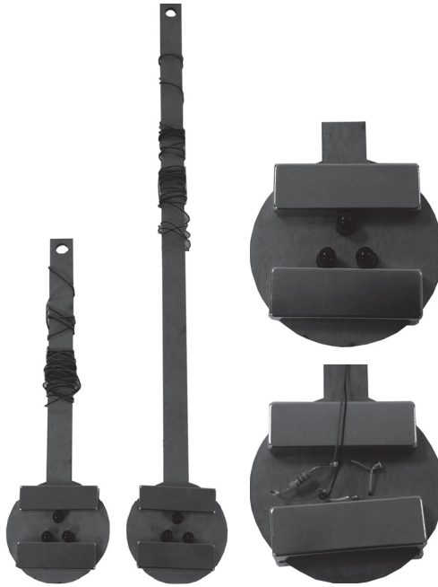
Figure 7.7: Pendulums laser cut from acrylic with integrated IR LEDs and added magnets for weight.
