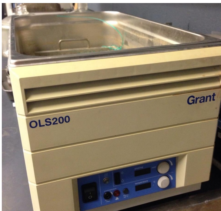
Figure B-1 Temperature-controlled water bath shaker
