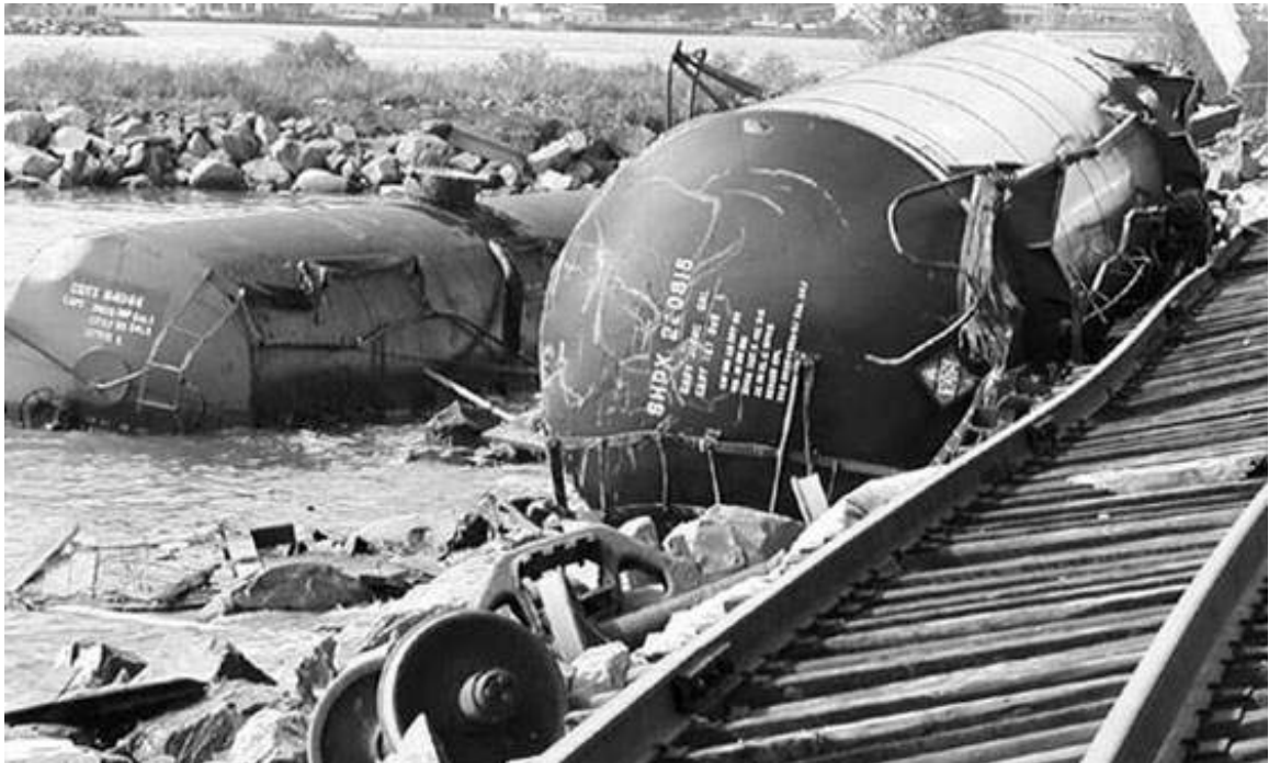
Photo 4.1: Rail cars and tracks washed out by Hurricane Juan storm surge (Environment Canada 2015b)
