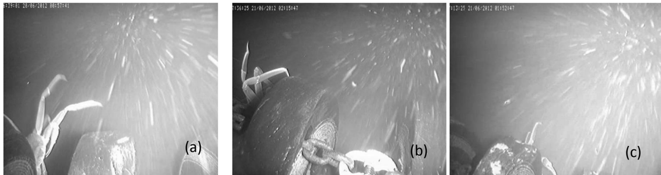
Figure 2.2: Example images showing different types of encounter. (a) the crab got stuck into the disc; (b) the crab was snagged into the spacer/chain; (c) the crab went under the disc.
