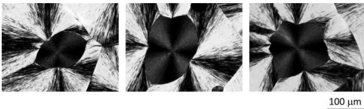
Figure 1. Examples of the morphologies obtained at the end of PPVL crystallization at 160 °C. Cross-nucleation of \alpha -phase can be observed at multiple points of the \gamma -spherulites periphery.
