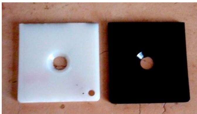
Fig. 3. Square specimen used for the tribological tests
