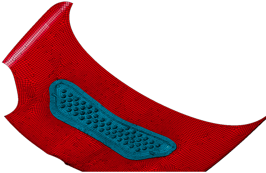
Fig. 8. Proposed prototype of the under-bonnet heat exchanger: both parts, upper part corresponding to the bonnet itself (in red, steel) and lower part (polymeric, in blue; to be bonded to the upper part).
