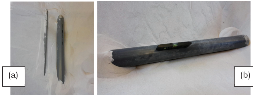
FIG. 8 – Second test set. PVC circular cylinders during burial: (a) cylinders #1 and #2; (b) cylinder #3.
