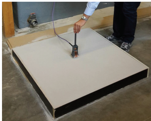
FIG. 2 – Measurements in small sand box with different volumetric water contents.
