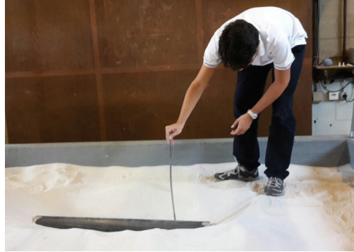
FIG. 4 – An empty PVC circular cylinder is being buried during the preparation of the test sets for the B-scans in the sand container.
