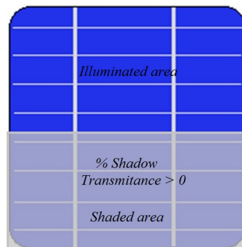
Fig. 3.6 Partially shaded PV cell
