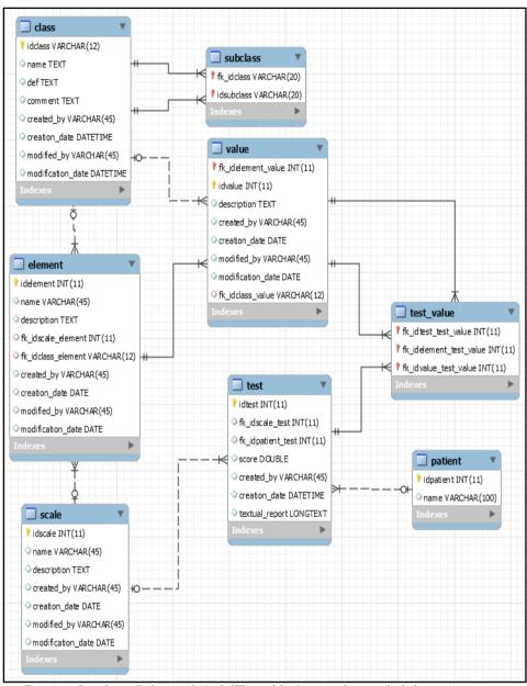
Fig. 4.1. Database Relational ModelThe table 'patient' recorded the patient identifier, the tables 'test' and 'test\_values' stored the information about the tests covered by the SARA, and the rest of the tables recorded the information modeled in the clinical archetypes.
