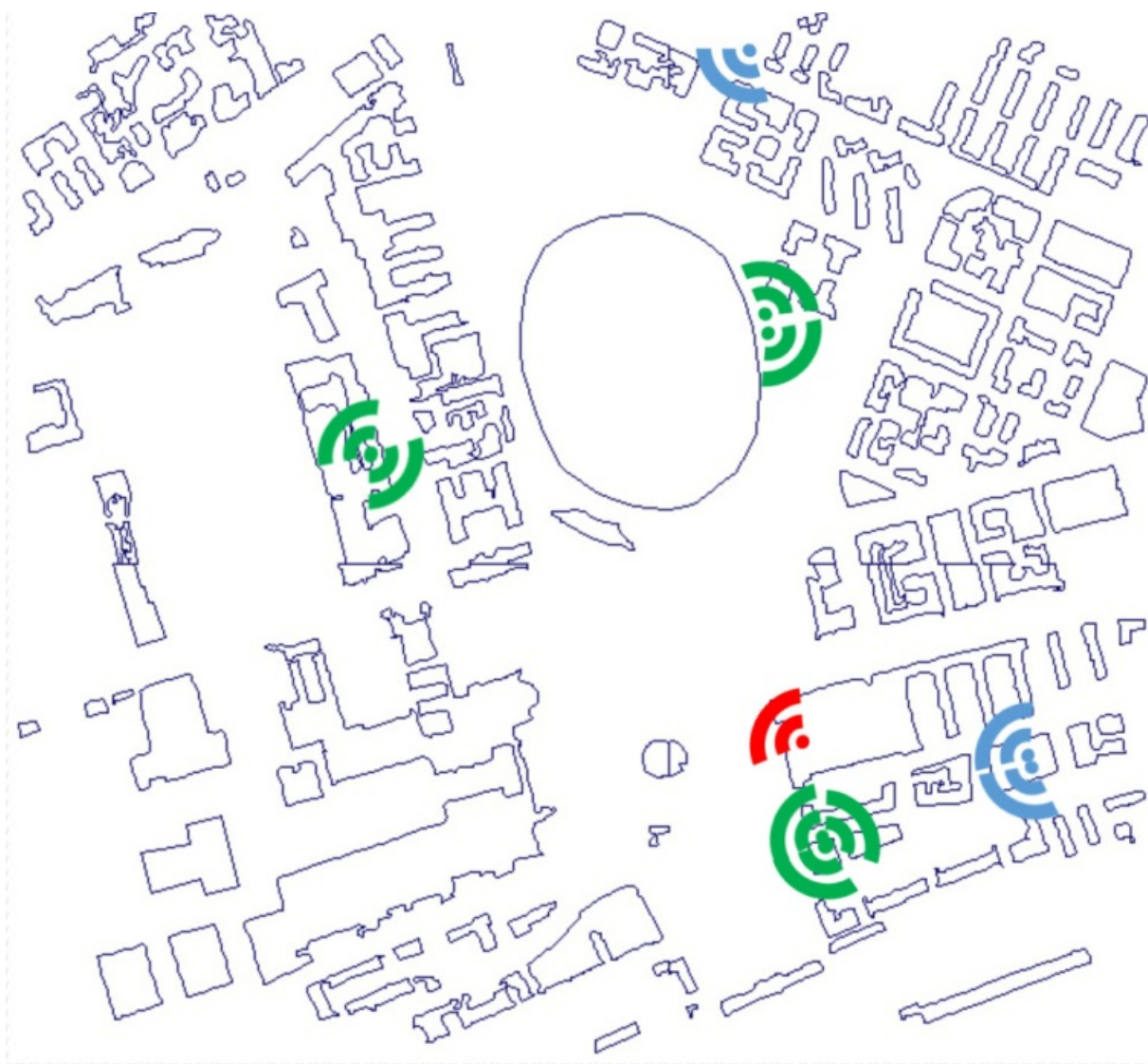
Figure 50: Map of the city (Fuorigrotta area) section with locations of transmitting antennas. Different colors refer to different telephone companies.
