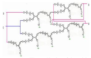
The combination of these delay flip flops will form the registers which is used for storage. The connections made here with lines are just for simplicity and to reduce the confusion in connection and in practical it should be formed with polyphenylene molecules as before.
