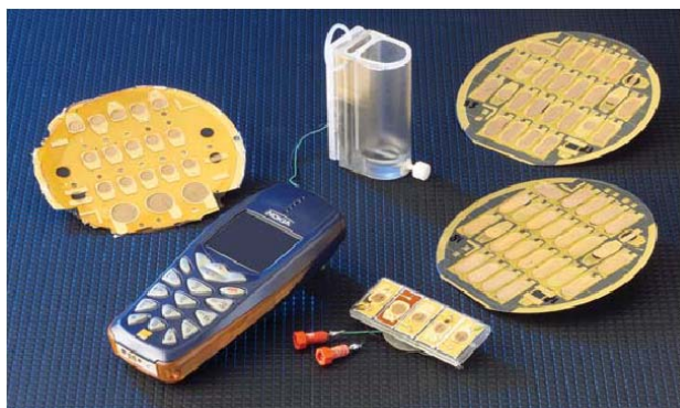
Figure 1: From the wafer to the phone, the fuel cells by the CEA after [20].
