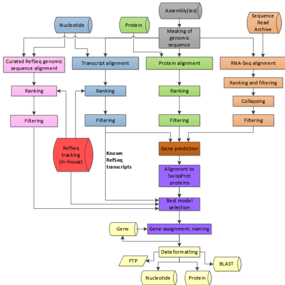
Figure 2. NCBI’s annotation pipeline to validate and annotate sequences shows how many different resources are pooled to develop a single consensus sequence and corresponding annotation (NCBI, 2016).
