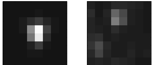
FIG. 12.— Synthetic images produced from the pixel-response function (PRF). Left .—A target star. The PRFs computed for 9 wavelengths have been stacked to form a single image. The weight of each PRF in the sum depends on the stellar effective temperature. Right .—Fainter stars in the vicinity of the target star. We sum the flux from neighboring stars, with PRFs weighted according to the T_{\text{eff}} of each star, in the same fashion as the target stars.
