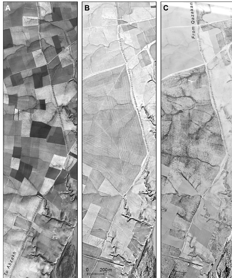
Fig. 8 - The Qazakan-Abzakh subterranean channel, visible by the alignments of collapsed access shafts (dark spots). A. U2 mission 1554 (29 January 1960). B. HEXAGON mission 1213 (14 November 1977). C. HEXAGON mission 1214 (2 May 1978). See also Fig. 2 for Jones' map of this feature.
