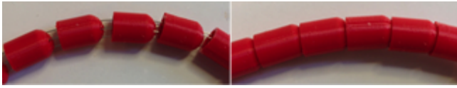
Fig. 2. (left) Vertebrae are connected in series by pull wires; (right) Pull wires are tensioned to lock vertebrae in place.
