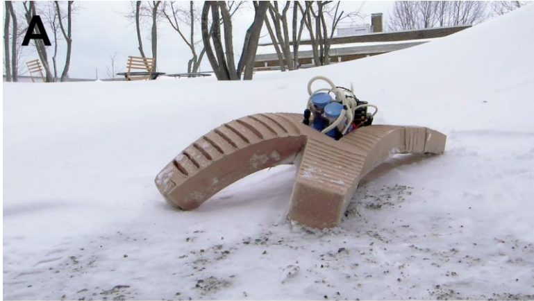
Figure 4. Resilience of the untethered soft robot to harsh conditions. (A-C) Images from experiments of the soft robot operating untethered in a variety of harsh conditions, including a snow storm (A), a fire (B), and water (C).
