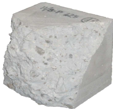
Fig.19 - Sample P-18 after explosive spalling
