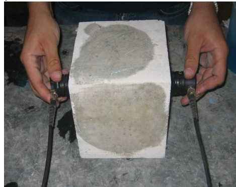
Fig.6 - Application of ultrasonic probes
