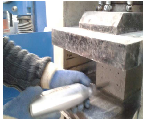
Fig.7 - Carrying over sclerometric tests
