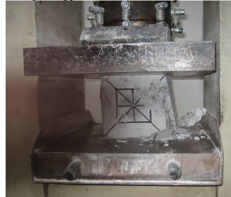
Fig.8 - Breaking specimen under crushing
