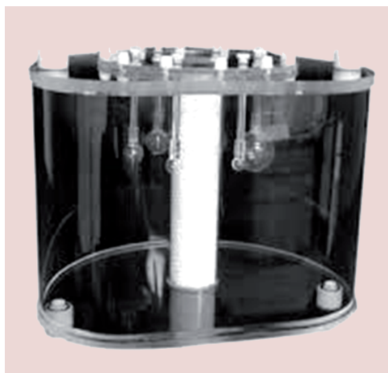
Figure 1. Image of the specific phantom utilized to perform PET/MRI acquisition of hybrid core shell nanoparticles. The low volume glass burettes are filled with a selected sample at a specific concentration.
