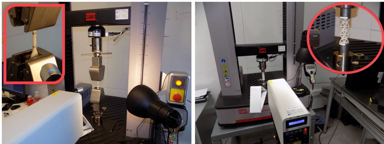
Fig. 5. 6 Right: Compression test setup on MTS C43 showing a laser extensometer, overhead light, and a video camera. A close-up of the cylindrical compression platens with the sample in place is shown in the top right corner. Left: Tension test setup. A close-up of the tension grips with the sample in place is shown in the top left corner.
