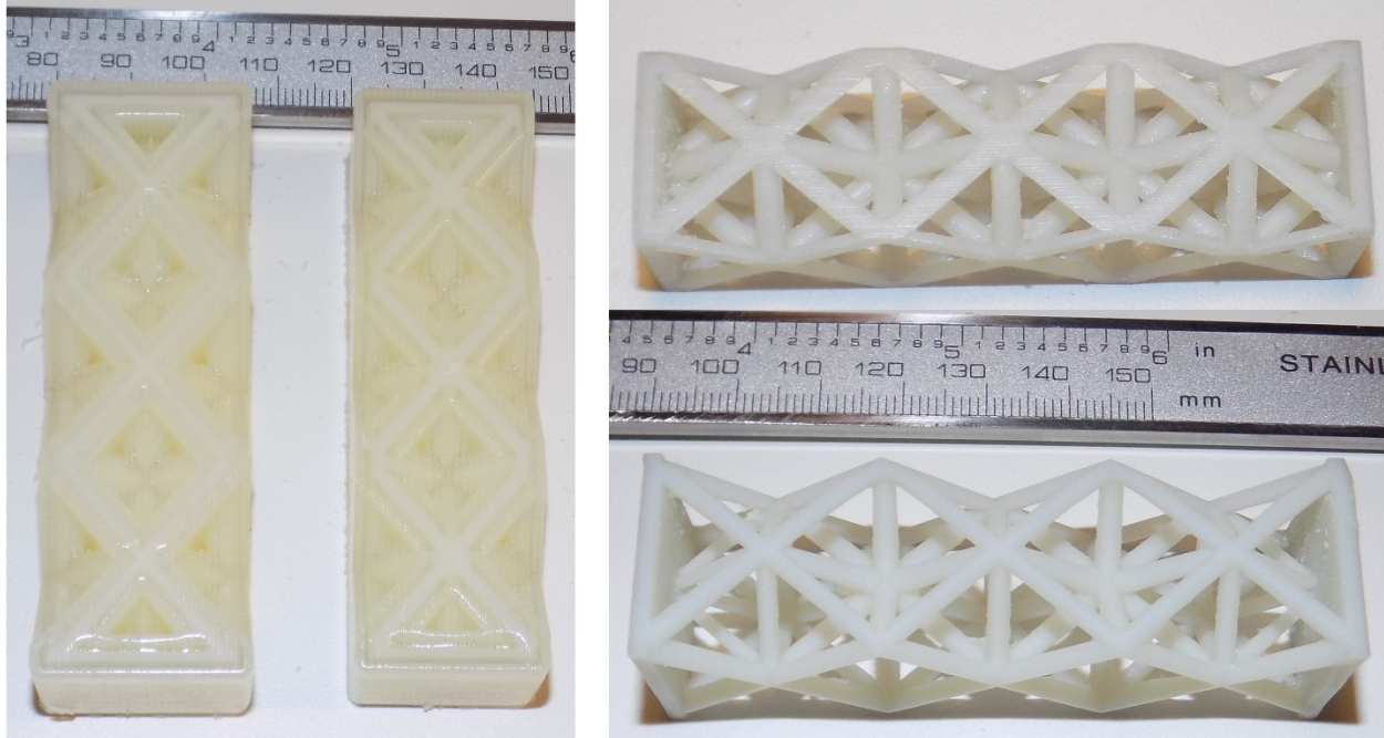
Fig. 5.8 Lattice structures generated using analytical model vs HyperWorks' LSO. Left: before removing support material (HyperWorks is left). Right: after removing support material (HyperWorks is bottom).
