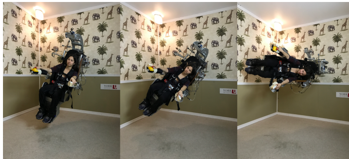
b) Naso-occipital rotation of built-in Tumbling Room Chair
