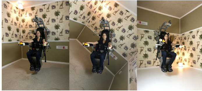
a) Naso-occipital rotation of Tumbling Room
