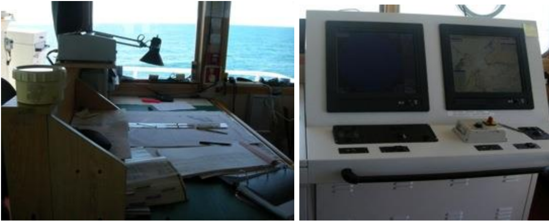
Image 5.8 a & b: The photograph on the left shows the paper sea chart and table. The photograph on the right shows the console featuring Radar (on the left) and ECDIS screen (on the right). Photos: 17 August 2010.
