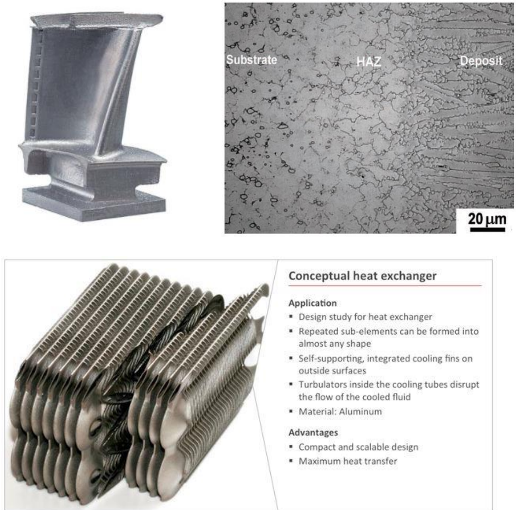
Figure 6 - Top left: turbine with cooling cavities [24]. Top right: “Optical micrograph of a CoCrMo LBMD deposit on a wrought substrate illustrating a refined carbide structure in the deposit and a small heat affected zone (HAZ)” [9]. Bottom: engine radiator [25].
