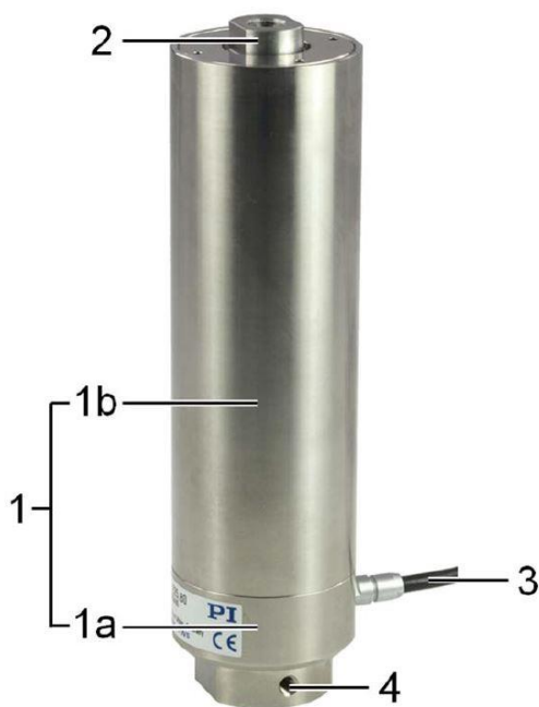
Figure 23 - Example of a piezo stack actuator (1 Case, consisting of: 1a: Base with wrench flat 1b: Case tube; 2 Moving pusher with wrench flat and M8 internal thread; 3 Cable exit for piezo voltage; 4 Protective earth connection) [18].
