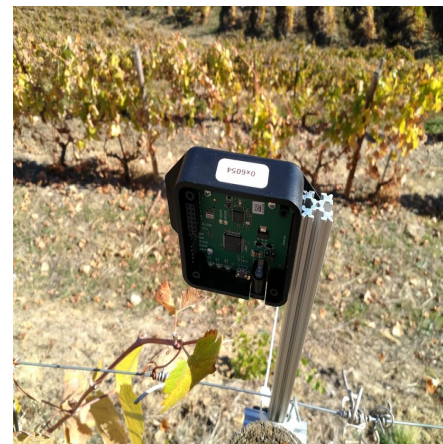
Figure 4.11: Beacon placement in a vineyard trellis
