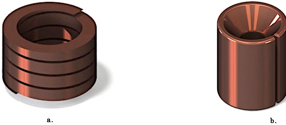
Figure 43: a. Primary coil; b. Fieldshaper (w/radial slit detail) developed.
