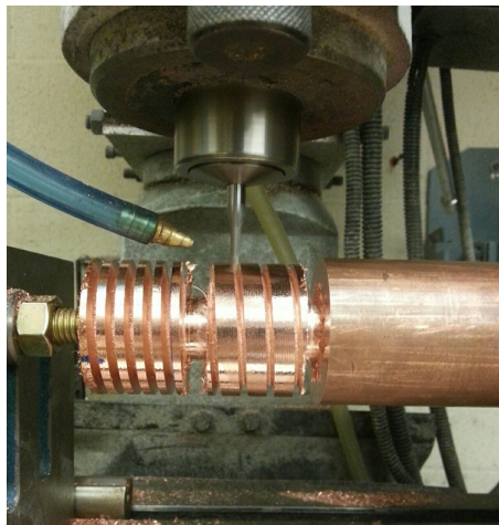
Figure 69: Manufactured coils. Left: Original design with 5.5 turns. Right: Alternative design with 3 turns.
