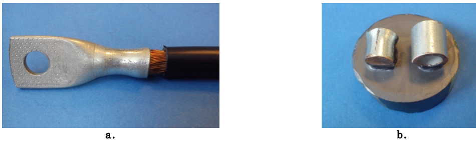
Figure 40: a. Detail of the modification of surface finish after compression b. Samples prepared for SEM observation.
