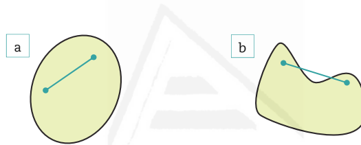
Figure 2.10. Example of (a) convex and (b) nonconvex sets.
