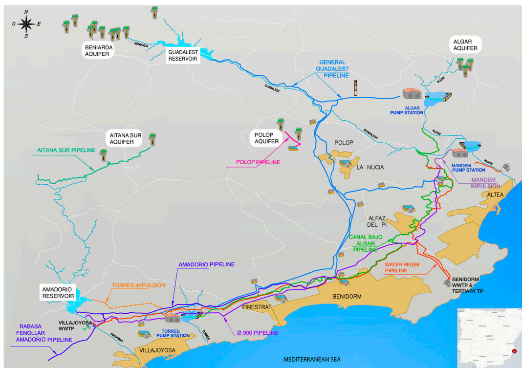
Figure 1. Map of water supply system in Benidorm and the Marina Baja Region (Source: Adopted from Marina Baja Water Consortium).
