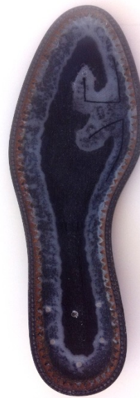
Figure 13: Shoe sole with adhesive applied.
