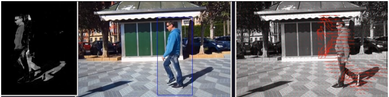
Fig. 4. From left to right: Sum of subtracted frames, detected pedestrian, Optical flow, a video showing an example of the preprocess input video stream can be found at: https://youtu.be/5dN4oePAqTg
