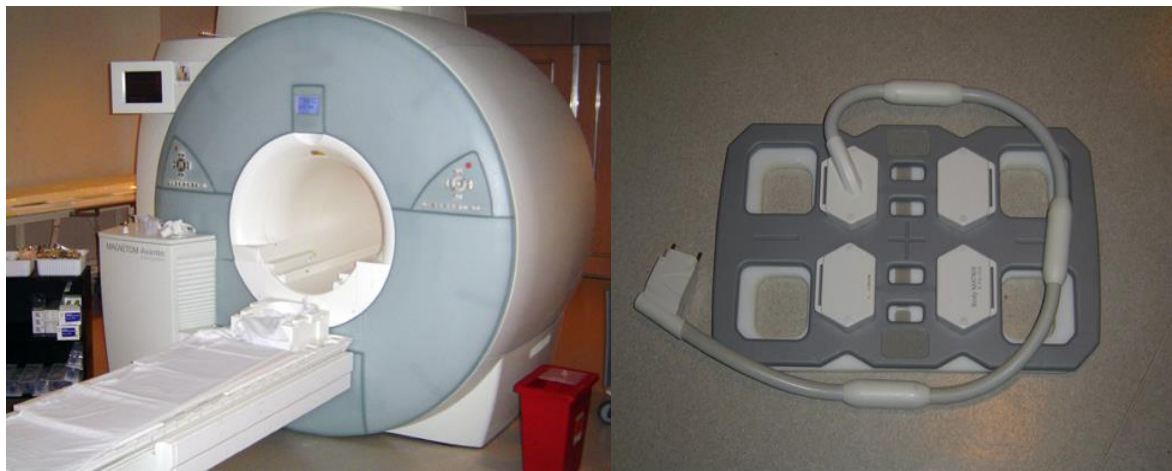
Figure 2.19: 1.5 T MRI scanner used in cardiac MRI (left) and a RF coil (right) to be placed on the patient's chest during MRI scan. Adapted from [46].
