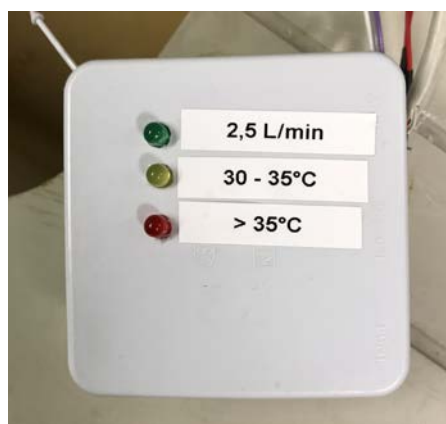
Figure 7.13 – Warning lights system
