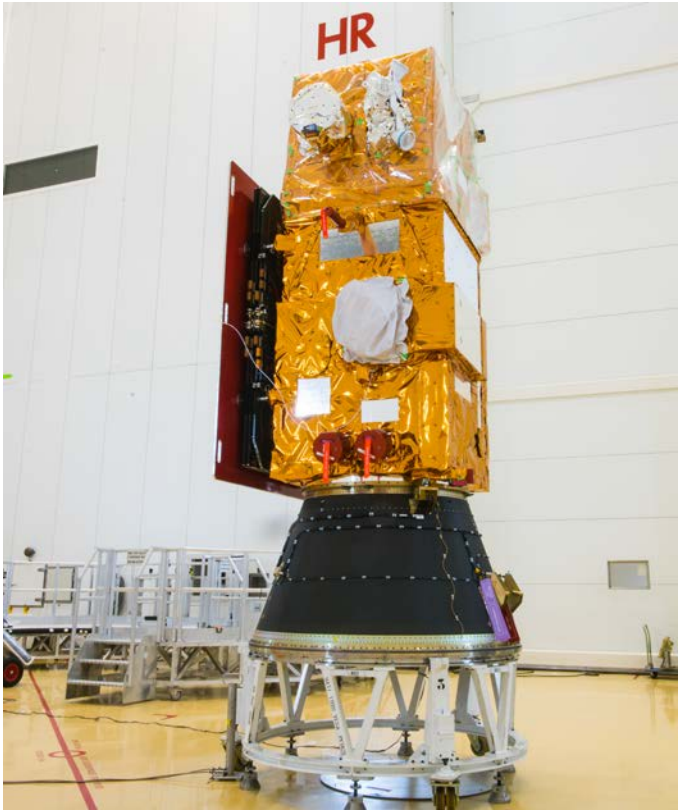
Figure 2.2 - Sentinel-2B installed on its payload launcher adapter (courtesy of ESA)
