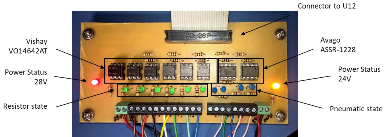
Figure 7.7 – Board Control final result. All components soldered and operational.
