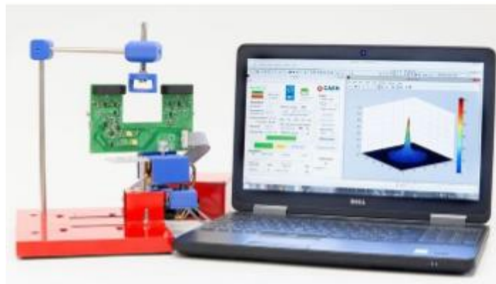
Figure 7.2: Image used for commercial purposes by Caen, portraying the U-shape PCB with two detectors, one at each U-tip [37].
