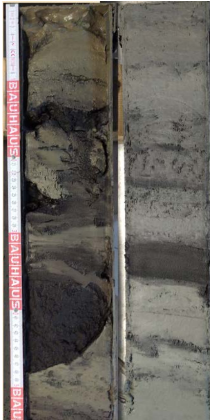
Fig. 1: Core of station 3. (left) Topmost 60 cm showing the major volcanoclastic turbidite above a steep erosional unconformity (48 cm bsf) and with a m \acute{e} lange-like mixture 15-28 cm bsf. (right) Segment 100-155 cm bsf showing an apparently compositionally zoned ash bed with a gray lower layer and a black main part around 135 cm bsf.
