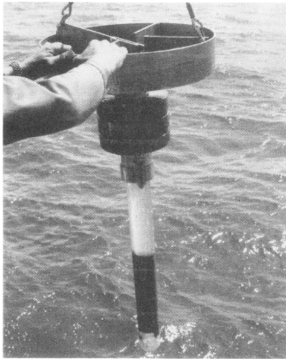
Fig. 4. View of a modified Meischner & Rumohr (1974) gravity corer after collecting an undisturbed sediment core.
