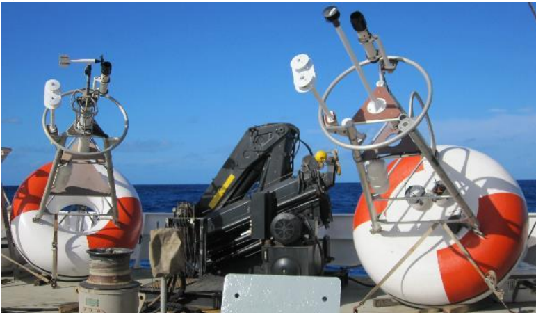
Fig. 3. a) Old buoy on the left and new T-Flex buoy on the right b) submarine part of the existing CO 2 sensor installed on an old buoy.
