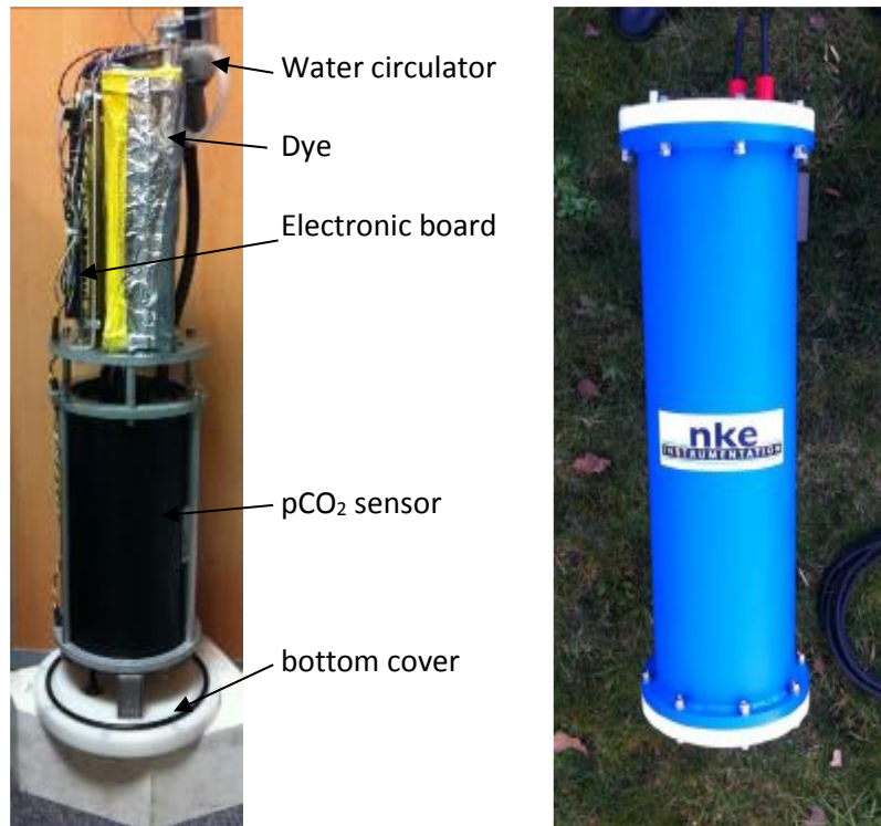
Fig. 4. Submarine part built by NKE for the T-Flex buoy at 6°S, 8°E.
