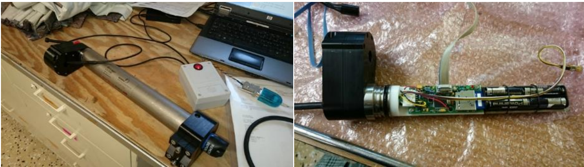
Fig. 1: (a) O_2 sensor consisting of Aanderaa oxygen optode (here: model type 4330) and logger unit including the inductive modem module (IMM). (b) Interior of logger unit and IMM.
