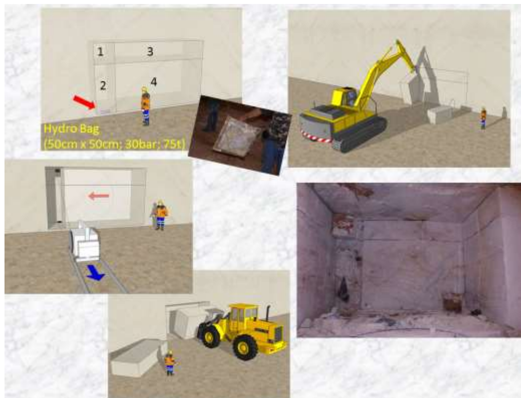
Figure 12 –Gallery advancement made using the decentered cross technique. Original draws by Emanuel Branco.
