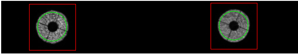
Figure 7. Configuration of the TP3-WFS, represented over an actual image read from the WFS camera while pointing to a natural star. The red squares correspond to the extracted pupil regions, while the green circles represent the size of the Zernike functions used for precalculating the slope maps. The background image does not correspond to a full frame but to a limited number of scan lines, in an attempt to maximize the camera sampling rate by reading only the region of interest.
