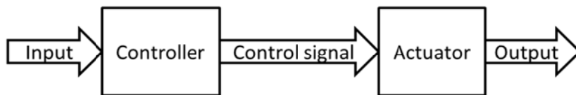
Figure 1: Scheme of an open-loop control system.
