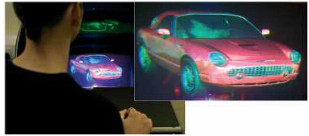
Fig. 5. Replay of a spatial-multiplexed, 3 \times 8 billion-pixel, full-parallax, full-color, 3D image [102]. (Slinger, C., Cameron, C., Stanley, M., "Computer-Generated Holography as a Generic Display Technology," Computer , vol.38, no.8, pp. 46–53, Aug. 2005. © 2009 IEEE. Reprinted with permission.)
