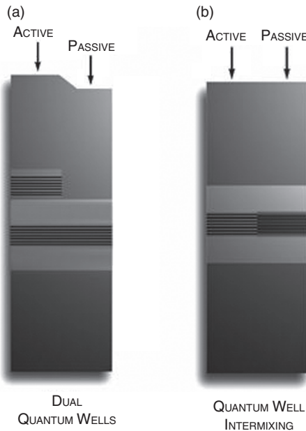
Figure 12.2. Schematics for (a) dual quantum wells and (b) quantum well intermixing methods [4].
