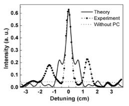
In order to investigate the subwavelength resolution, we use the same photonic crystal structure and first consider two coherent sources which are separated by a distance of  $\approx \lambda/3$  and placed 0.7 mm away from the photonic crystal interface. Figure 13a shows the lateral profile of the transmitted power 0.7 mm away from the second interface. There's a
