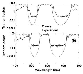
Figure 2 Measured (solid lines) and calculated (dotted lines) transmission spectra of CMC structures with intercavity distance  $\Lambda_A = 2.5$  (top) and  $\Lambda_B = 3.5$ , respectively
