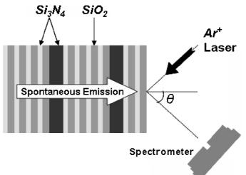
The room temperature photoluminescence (PL) measurements were performed using a 1-m double monochromator, equipped with a cooled GaAs photomultiplier tube and standard photon counting electronics, at  $\theta = 0^{\circ}$  with respect to the surface normal and with a spectral resolution of 2 nm. An Ar<sup>+</sup> laser operating at 488 nm with 120 mW output power was focused with a 15-cm focal-length cylindrical lens on the sample. The transmission spectrum is obtained by a fiber spectrometer.
