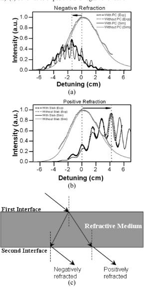
For the selected frequency, the incident field couples to the first band and propagates according to its dispersion. The advantage of the first band is that since  $\lambda > 2\sqrt{2}$  a the propagation does not suffer from Bragg reflections that take place inside the photonic crystal and we have a well defined single beam propagation. For this reason Snell's law
