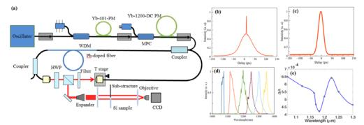
**Fig. 1** (a) The schematic of experimental setup. WDM, wavelength division multiplexer; HWP, half wave plate; MPC, multimode pump-signal combiner; T stage, translation stage Measured intensity autocorrelation (b) before and (c) after synchronization. (d) Measured different wavelengths. (e) Measured refractive index difference between silicon and modified silicon for different wavelengths.
